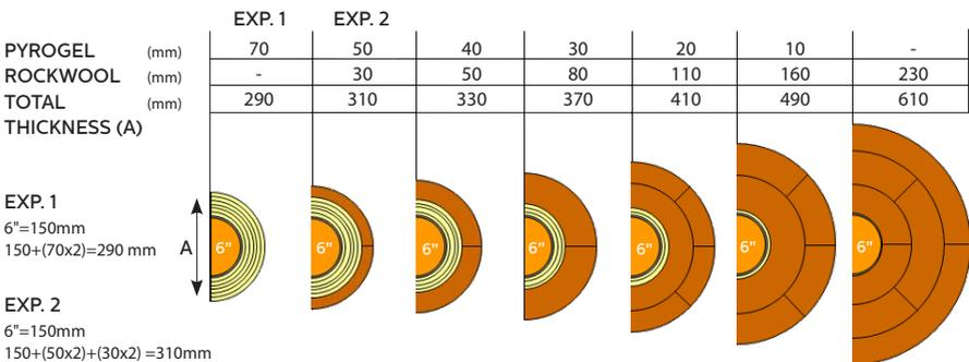
In this example, Pipe Size is 6", Pipe Inlet Temperature  $T_{in} = 550\text{ }^{\circ}\text{C}$ , Ambient Temperature  $T_{AMB} = 20\text{ }^{\circ}\text{C}$  and insulation surface temperature  $T_{SRF} = 40\text{ }^{\circ}\text{C}$ .
