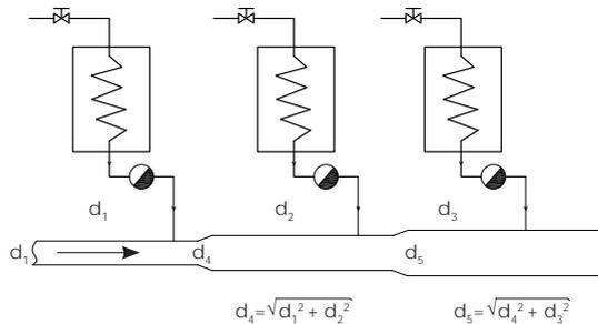
10- Steam traps must never be connected one after another in any case. Otherwise, first steam trap is affected negatively from the back pressure generated by the second steam trap.
