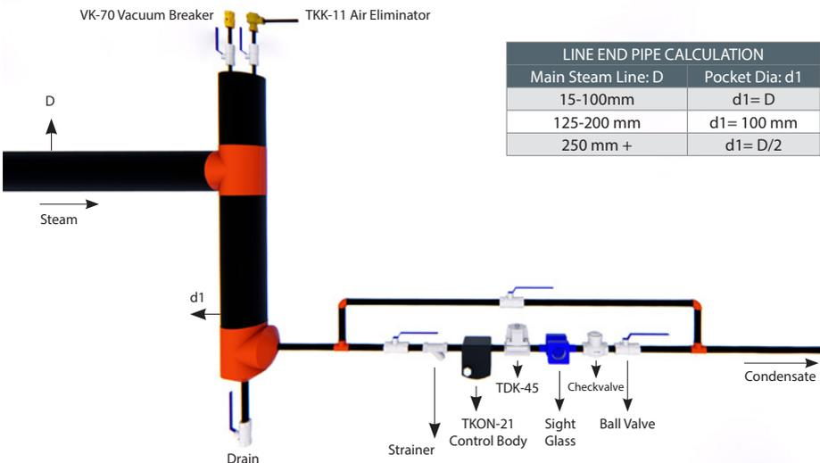
The system that distributes steam is called “**collector**”. Steam condensates in the collectors. The condensate is usually charged by thermodynamic steam traps from the collectors.
