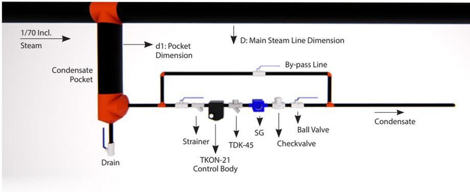
The occurred air and condensate around connection areas in the pipelines are dragged to the end of the line. If that air and condensate are not discharged, they may block the steam flow. In such cases, formed air and condensate are discharged with a line end application shown below. The steam trap kind must be thermodynamic.
