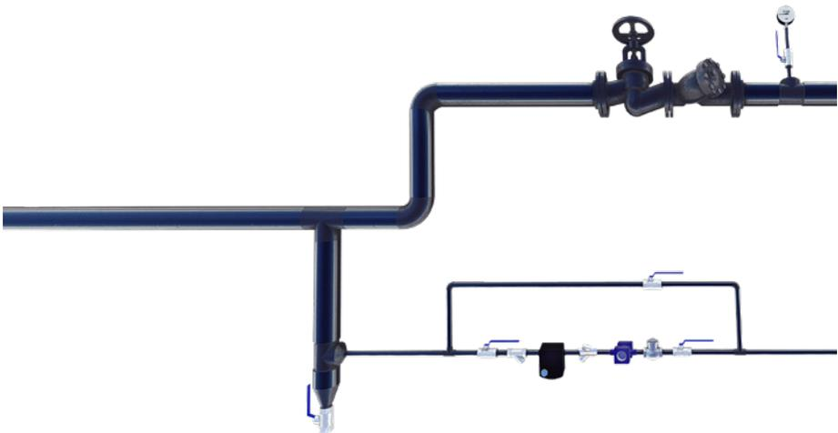
Branch lines to the steam equipment should not be taken from the bottom or side walls of the main lines because of the formation of dirt or residues. Branch lines should always be taken from the top of the main steam lines.
