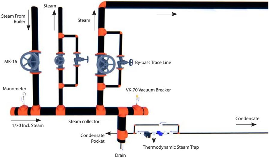
In cases where dry and clean steam is required, branch line should be connected to the machine and process with a steam separator. This will help to collect the water at the bottom of the separator and to be discharged from the steam trap.
