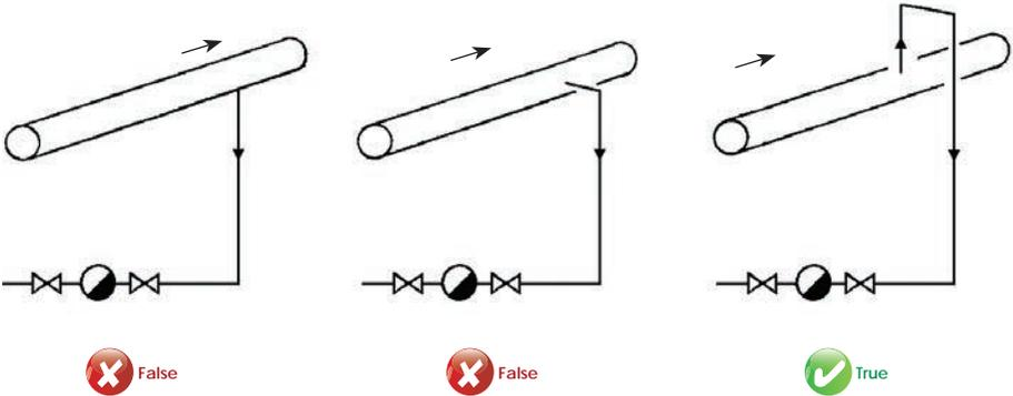
If any elevation in the pipeline after the boiler is applicable, the pipeline diameter of the elevated area is built bigger. That helps to reduce the speed of the condensate and flows back to the discharge unit. In elevating parts of the pipelines, creating condensate discharge units in every 15 meters is advised.
