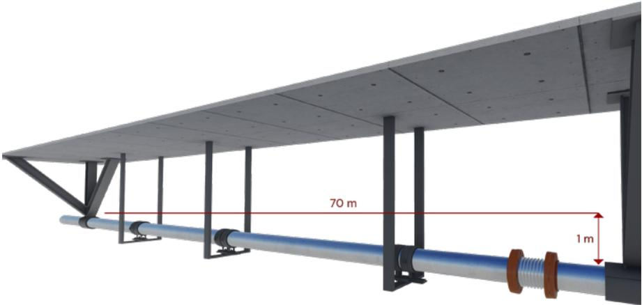
The points where the main lines are elevated, condensate collecting pockets should be created at the bottom turning points and thermodynamic steam traps to be placed.
