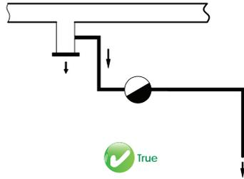
11- In examples where the condensate is pumped to the condensate tank, hot condensate outlets from the steam trap connects the cold condensate and means serious water hammering risk to the system. In these cases, there must be at least 5 meters of distance between the main condensate line and the line after steam trap.
