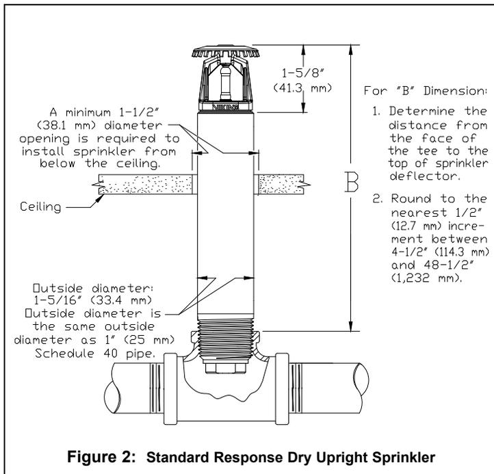
Figure 2: Standard Response Dry Upright Sprinkler
