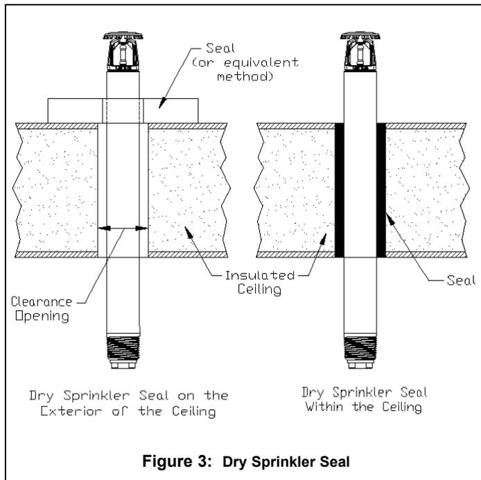
Figure 3: Dry Sprinkler Seal
