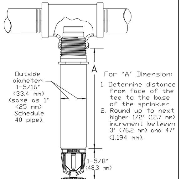
Figure 5: Plain Barrel Dry Pendent Sprinkler
