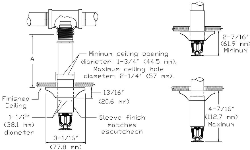
NOTE: To locate the deflector at the minimum distance below the ceiling, with no upward adjustment available, order the dry pendent sprinkler 1" (25.4 mm) shorter than the A dimension.
