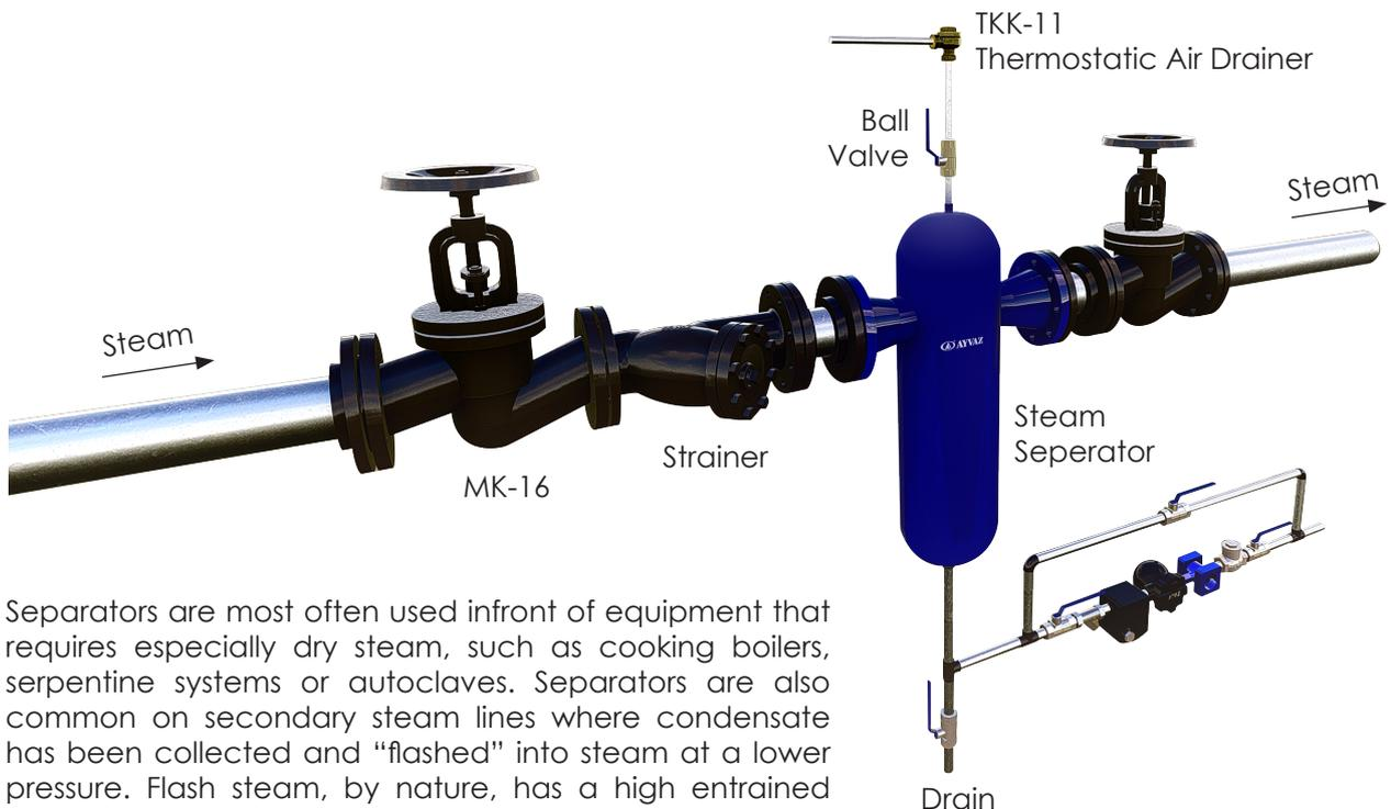
Separators are most often used in front of equipment that requires especially dry steam, such as cooking boilers, serpentine systems or autoclaves. Separators are also common on secondary steam lines where condensate has been collected and “flashed” into steam at a lower pressure. Flash steam, by nature, has a high entrained condensate content.
