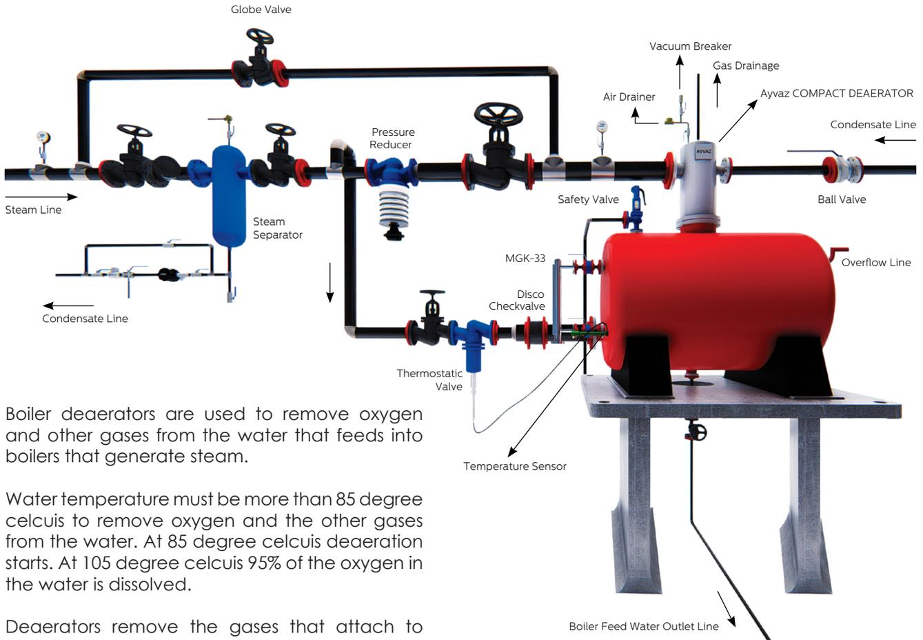
Boiler deaerators are used to remove oxygen and other gases from the water that feeds into boilers that generate steam.
