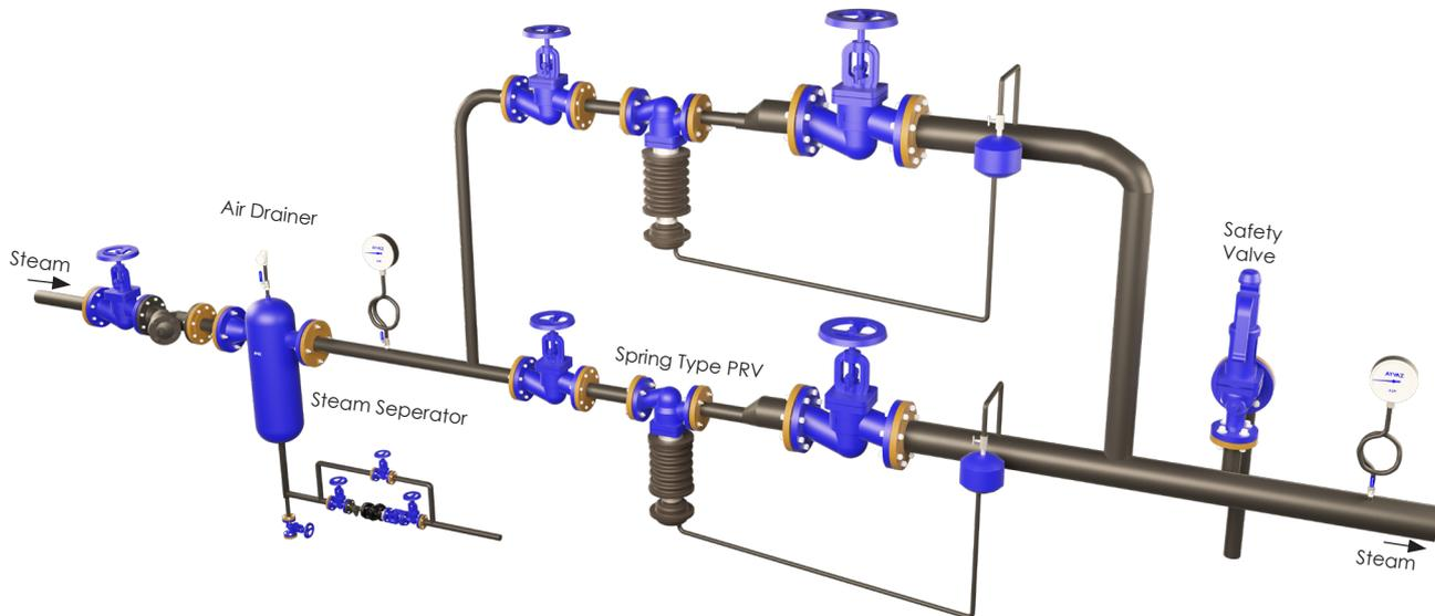
The choice of the main pressure reducing valve must depend on the needs of the system. In a folding machine where the same pressure is always required in high temperature cylinders with a very stable demand throughout the process, a direct effective pressure reducing valve of the correct size can be safely used.
