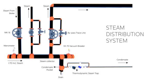
The system that distributes steam is called "collector". Steam condensates in the collectors. The condensate is usually charged by thermodynamic steam traps from the collectors.
