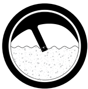
Figure B/Normal Operation The deflector below sight axis, there is no steam leak, the steam trap is operating normally.
