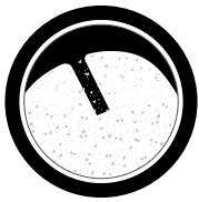
Figure C/Condensate Water Accumulate If the flow indicator is completely covered by water, it must be understood that the sight glass installed very close to the system and there is condensate accumulation in the device with heat transfer. As the result that the steam trap capacity is insufficient.
