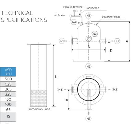
**Design Pressure:** 5 bar **Design Temperature:** 198°C
