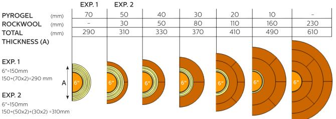
In this example, Pipe Size is 6",  $T_{in}$  = 550 °C ambient temperature  $T_{AMB}$  = 20 °C and insulation surface temperature  $T_{SRF}$  = 40 °C.
